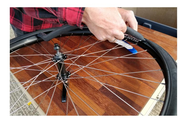
It is important to inspect the tyre before installing the new tube. The cause of the flat, such as a nail, thorn or piece of glass, may still be embedded in the tyre or tread. Inspect both the outside of the rubber tread and the inside of the casing removing any objects where necessary.
