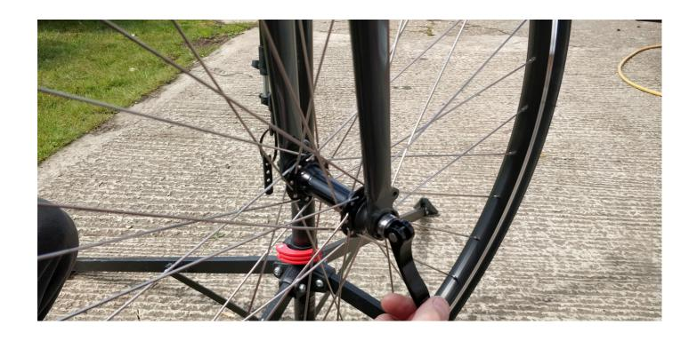
Disengage the Wheel from the frame by pulling the quick release skewer lever. If necessary, loosen quick-release adjusting nut to clear any tabs at the end of the fork.
