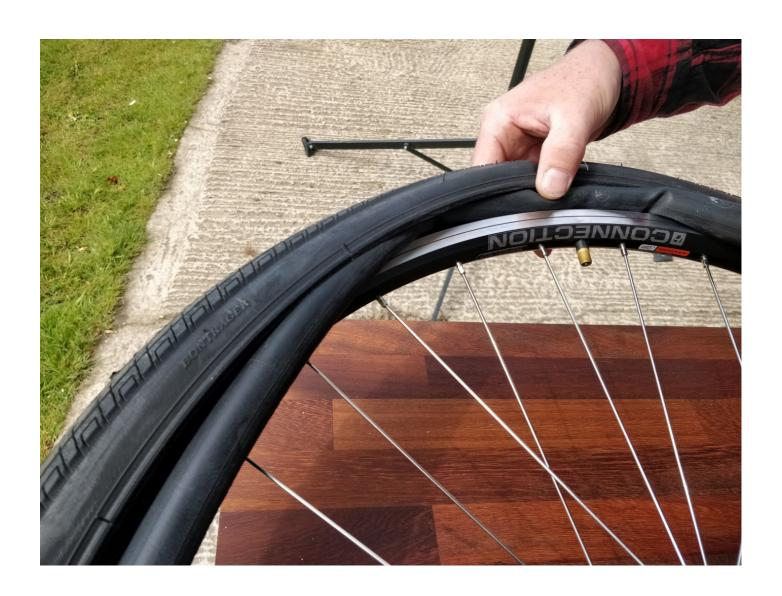
Install one bead at a time. Work tyre bead onto rim with hands. If the tyre bead will not seat by hand, use the tyre lever as a last resort. Use caution when using tyre levers to avoid pinching the inner tube. Engage tyre lever using same orientation as removing bead.
