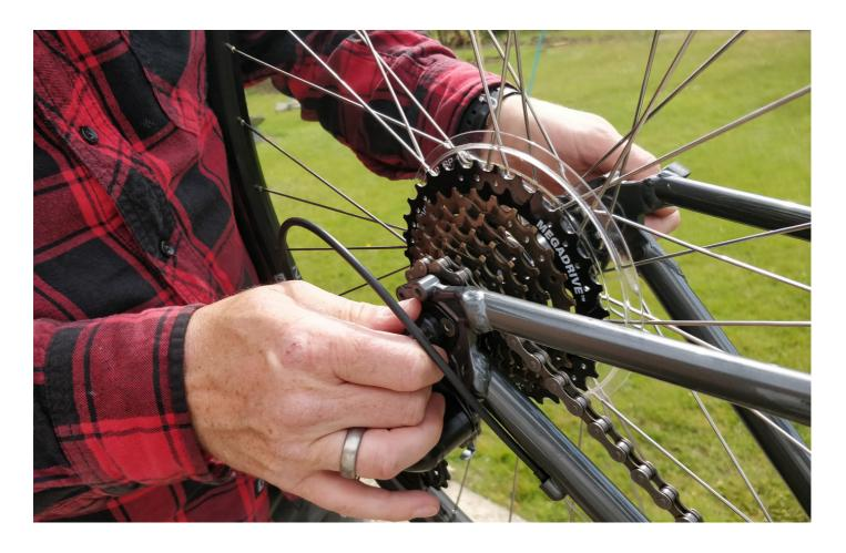
Tighten the Quick-release axle so that the lever meets resistance at 90° from the frame or fork.
