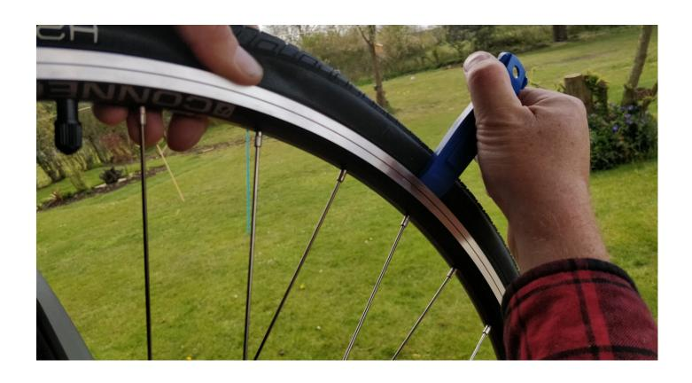
Inflate to low pressure and inspect the bead again on both sides. If beads look aligned correctly inflate to full pressure using the hand pump.
