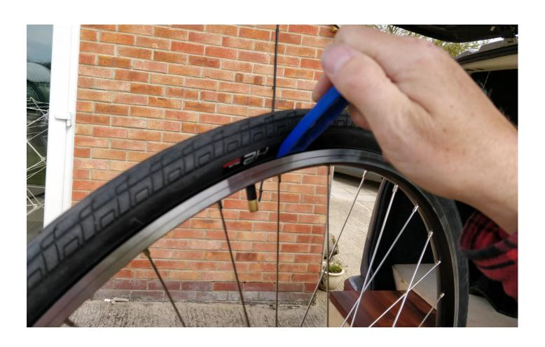
Starting opposite the valve, pull the inner tube from tyre. Lift valve from valve hole and remove tube from the wheel.
