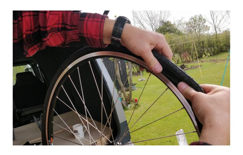
Work tube over rim sidewall and into rim cavity. Install second bead onto the rim.
