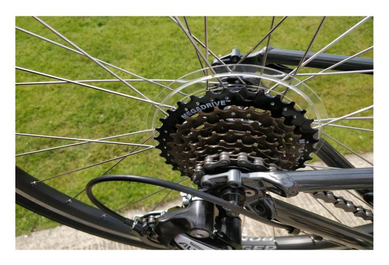
Disengage the Wheel from the frame by pulling the quick release skewer lever. If necessary, loosen quick-release adjusting nut to clear any tabs at the end of the fork.
