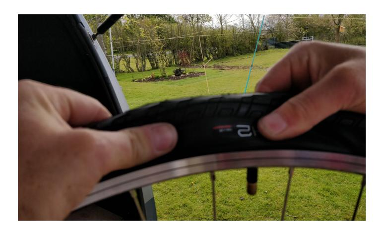
Engage one tyre lever under the bead of tyre. Engage the second lever 1-2" (25-50mm) from the first lever then pull both levers toward spokes to lift the bead off the rim. Disengage one lever. Move it two inches (5cm) along the rim and engage the lever in the bead. Pull lever to lift the next section of bead off the rim. Repeat engaging the lever until the bead loosens. Then slide the lever along the rim under the bead.
